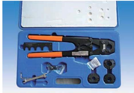
Crimp Tool 14" Length that crimps 3/8", 1/2", 5/8" and 3/4" copper crimp rings. For use on crimping PEX and Polybutylene Pipe with copper crimp rings. Includes Go-No-Go Gauge.
